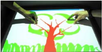
Figure 2. Image from the GroupLab Diamond Touch toolkit. MatchUs Board is a concept where two boards are individually used and are synchronized over net to provide a feeling of drawing something together and hence creating a shared experience. Image from, http://grouplab.cpsc.ucalgary.ca/software/DiamondTouchToolkit/index.html
